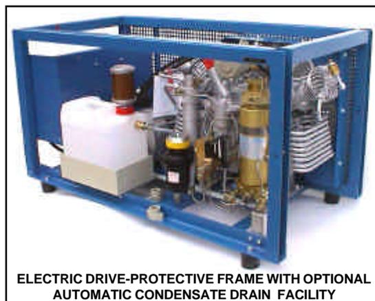
The electric models use a standard Molecular Sieve/ Activated Charcoal/Molecular Sieve format, whilst the Petrol and Diesel driven unit have an additional layer of Hopcalite catalyst to convert any traces of Carbon Monoxide to relatively harmless Carbon Dioxide.
