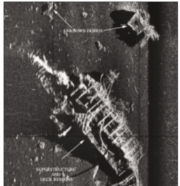
Figure 8: High-resolution sonar image of remains of Ark Royal superstructure (BBC and C & C).
