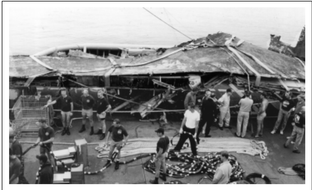
Figure 5-1. Starboard Wing Section. Large, jagged pieces of wreckage were difficult to rig, lift, and transport. Pictured above is an 80-foot section of the starboard wing aboard the USS GRASP.
