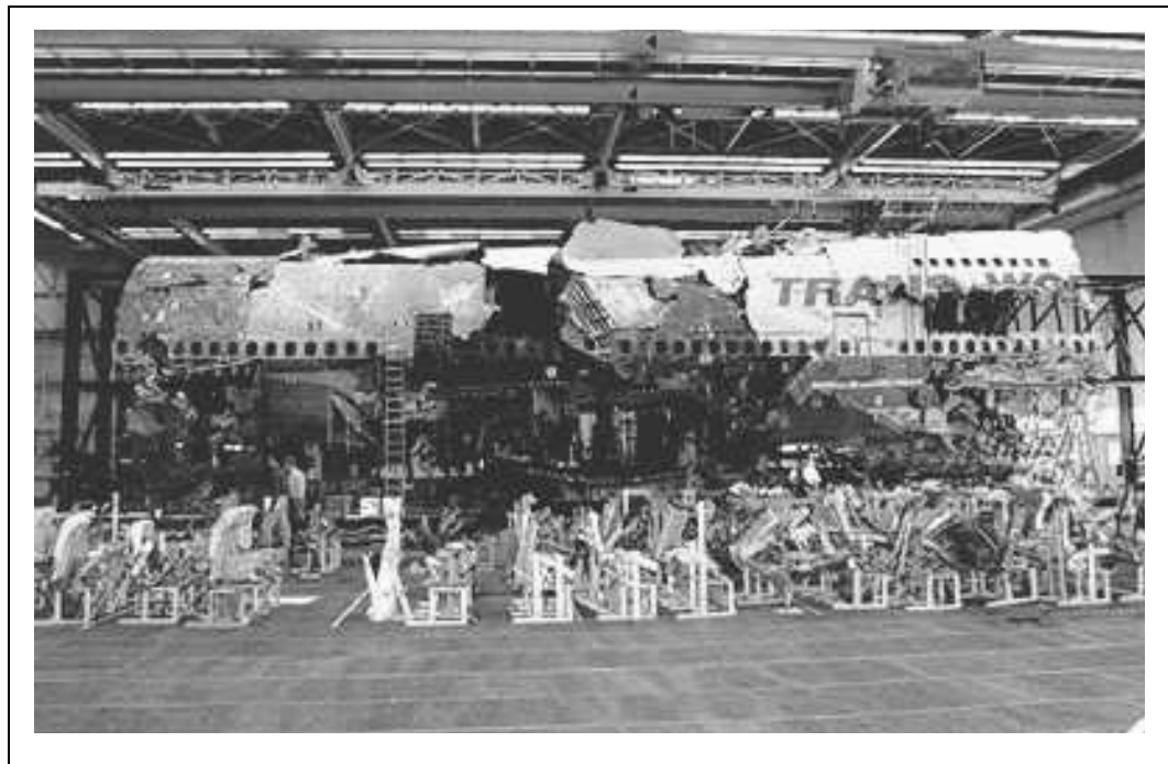
Figure 5-4. Reconstruction of Wreckage at Calverton Hangar. As part of its investigation, the NTSB used recovered wreckage to reconstruct portions of the aircraft. This photo shows a section of the fuselage, with passenger seats in the foreground.
