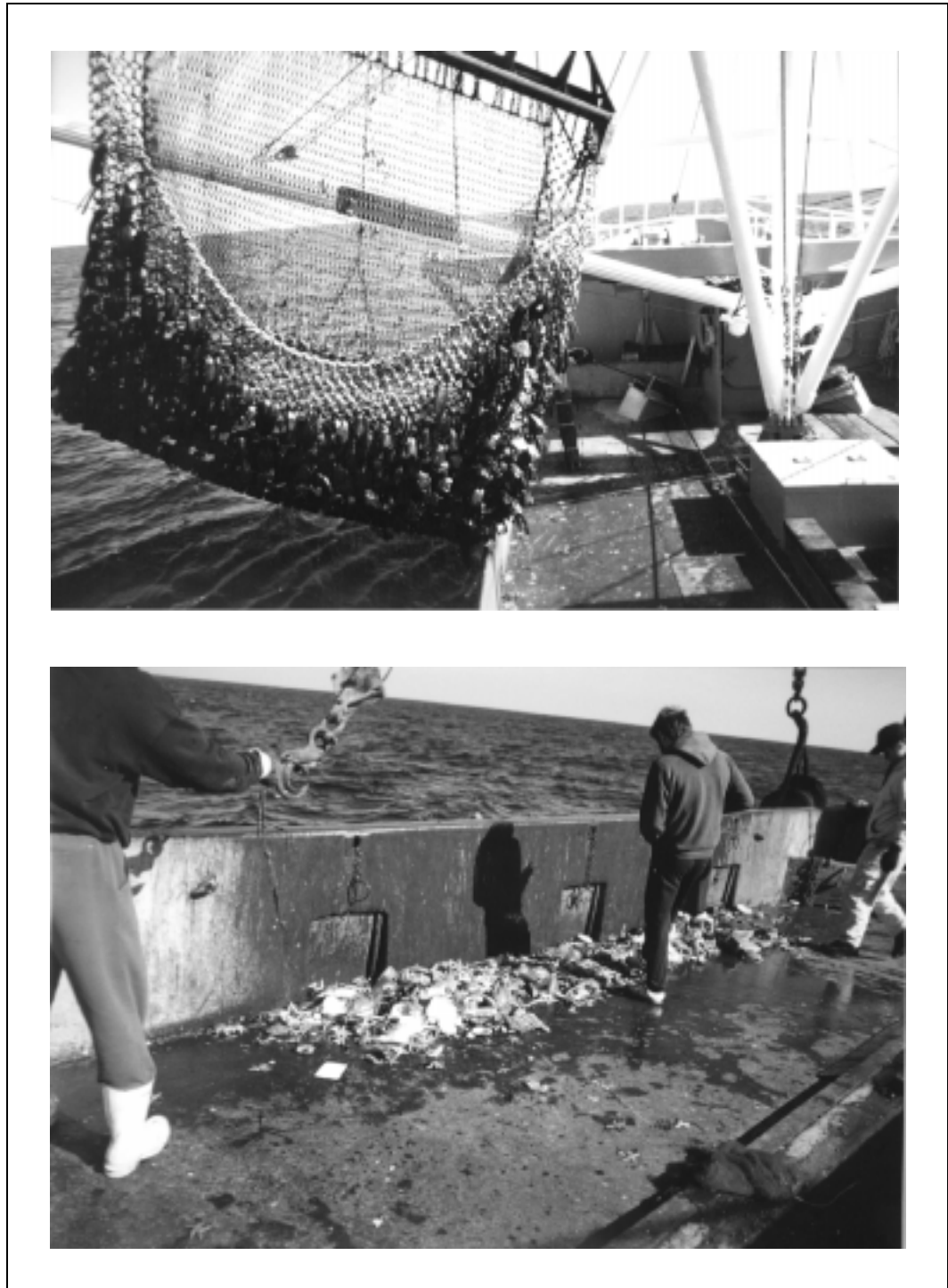
Figure 5-6. Trawling Operations. Top photo shows one of the 15-foot nets used for trawling. Bottom photo shows some of the small pieces of debris recovered from the ocean floor.
