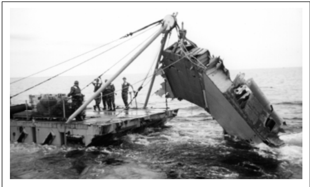
Figure 5-2. Tail Section. The Side Loading Warping Tug worked with the Mobile Dive Teams to recover large pieces of wreckage, such as this tail section.
