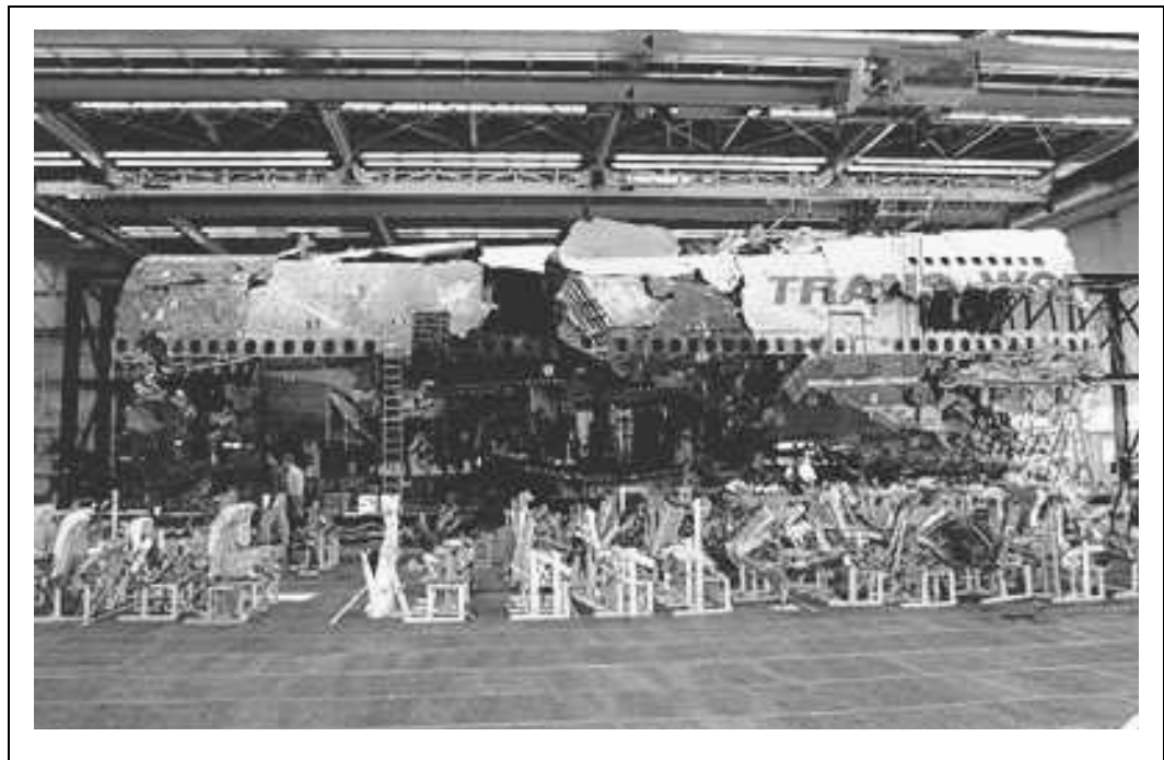
Figure 5-4. Reconstruction of Wreckage at Calverton Hangar. As part of its investigation, the NTSB used recovered wreckage to reconstruct portions of the aircraft. This photo shows a section of the fuselage, with passengers seats in the foreground.
