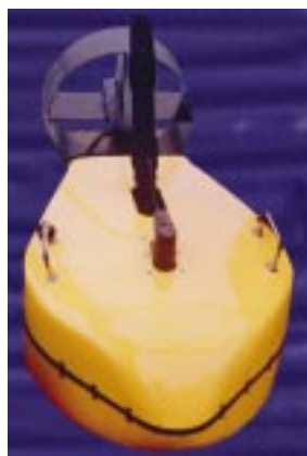
Model 400 Tow Vehicle with TC-2040 Transducers
